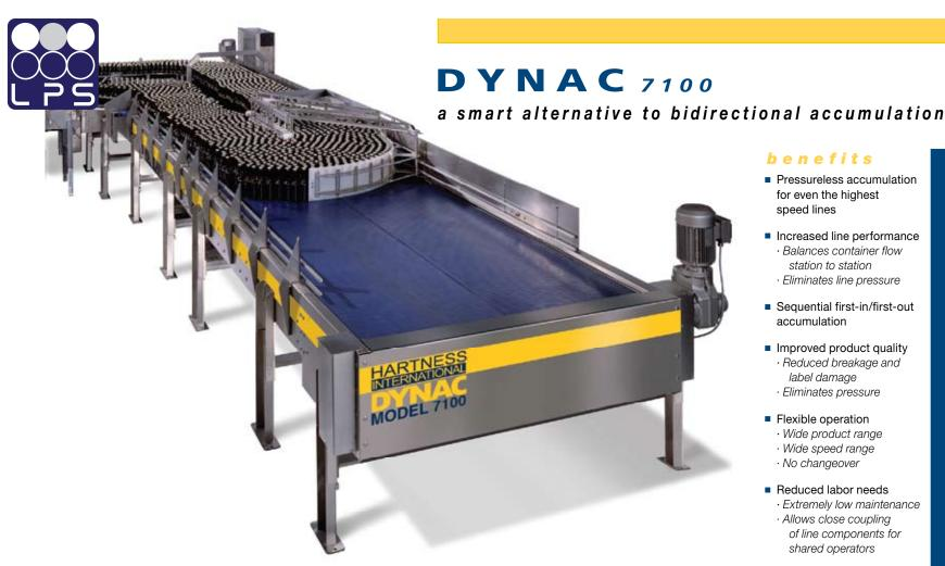
The Hartness Mass Flow 7100 DYNAC provides a much needed alternative to traditional high pressure accumulation systems.
